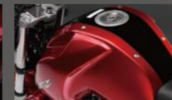
12-liter fuel tank with uniquely styled plastic resin cover
