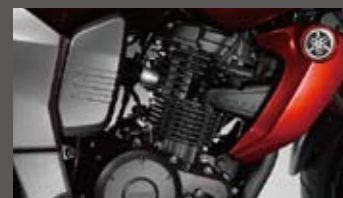
Air-cooled, 4-stroke, single-cylinder 153cc engine
